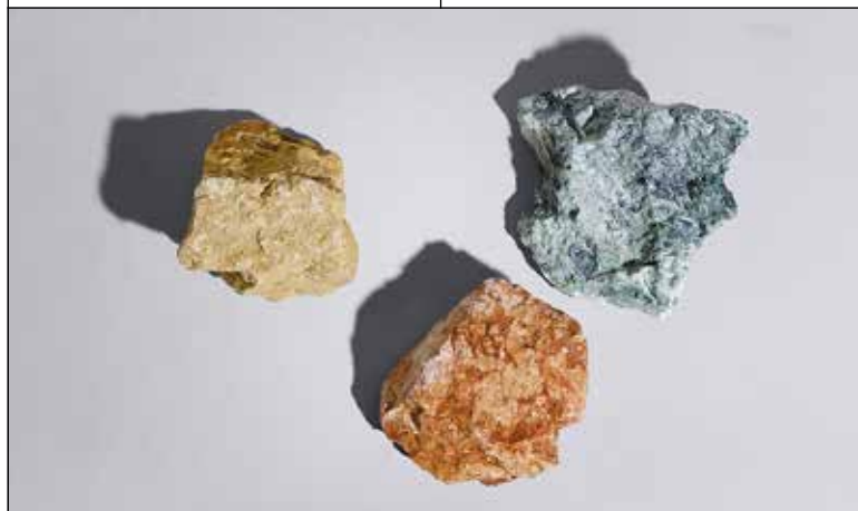
The Italian marbles used in Marmoreal: Giallo Mori, Rosso Verona and Verde Alpi
